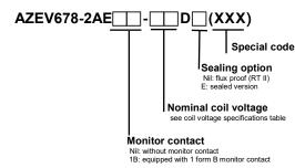
Note: For Ag plating contact (main load), add P after date code.
